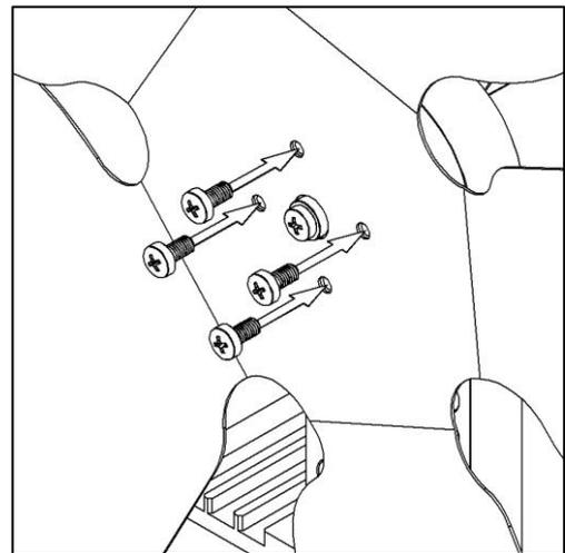
Fit fan blade onto hub and secure with 4 short screws.
