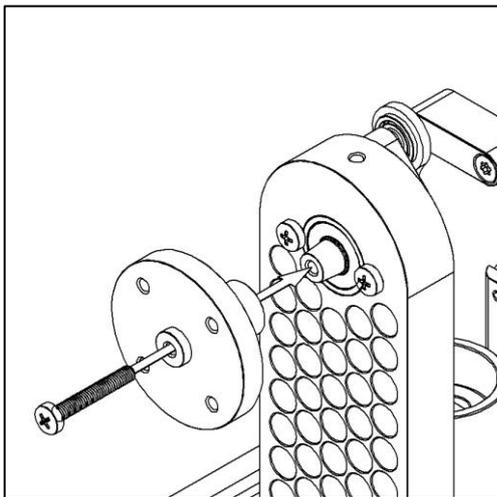
Fit hub onto axle and secure with 1 long screw.
